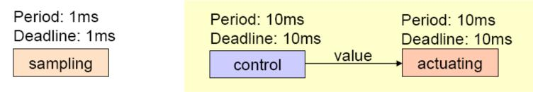
We must specify a precedence relation between the control task and the actuator task so that the control task always sends the latest calculated value to the actuator task
